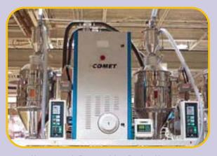
Honeycomb Dryer with 2 Drying Hoppers
