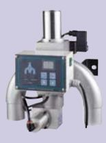
Comet's Two-Component CPV proportioning valve enables two materials to be conveyed in a preselected percentage through an individual hopper loader or a central vacuum receiver. Through in-line mixing, the CPV eliminates virgin and regrind layering, common in ratio loaders. Material proportion can be digitally set on the electronic control box mounted on the unit. During a single conveying cycle, it is possible to switch materials (virgin and regrind) as often as desired.
