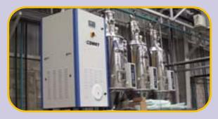
Centralized Honeycomb Drying System
