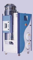
The compact dryer, mounted on a mobile frame, consists of three main parts: the Honeycomb Dehumidified Dryer, the Drying Hopper and the Loading System. The loaders feed to and from the drying hopper to the machine or, as an option, from the surge bin to the drying hopper. The FCD can supply one material to six machines and, depending on production requirements, special loaders can be designed to handle powder and dust separation. The vacuum pump and fines filter are mounted inside the unit.
